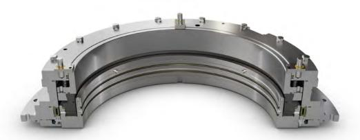
Axial type seals are typically used at hydroelectric power stations and municipal facilities, in turbines and pumps where higher pressures and more robust conditions prevail. Their main purpose is to maintain a near water tight seal between the shaft and the headcover of the unit.
